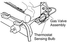
Figure 30 - Location of Gas Valve Assembly and Thermostat Sensing Bulb
